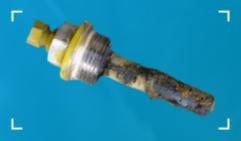
Clogged nozzles vapourise the odorant not sufficient anymore which leads to a higher consumption.
